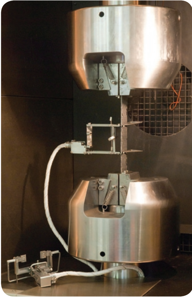
Elevated tensile using high-heat extensometers for Poisson's Ratio.
