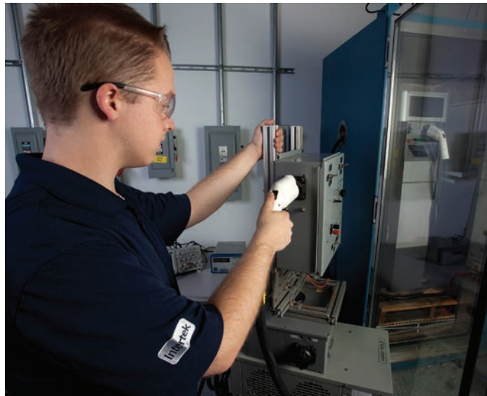
Engineer Nick Van Klompenberg of Intertek tests the safety circuits within an EVSE, using custom-fabricated test fixtures capable of simulating various environmental and fault conditions that may be seen in the real world
