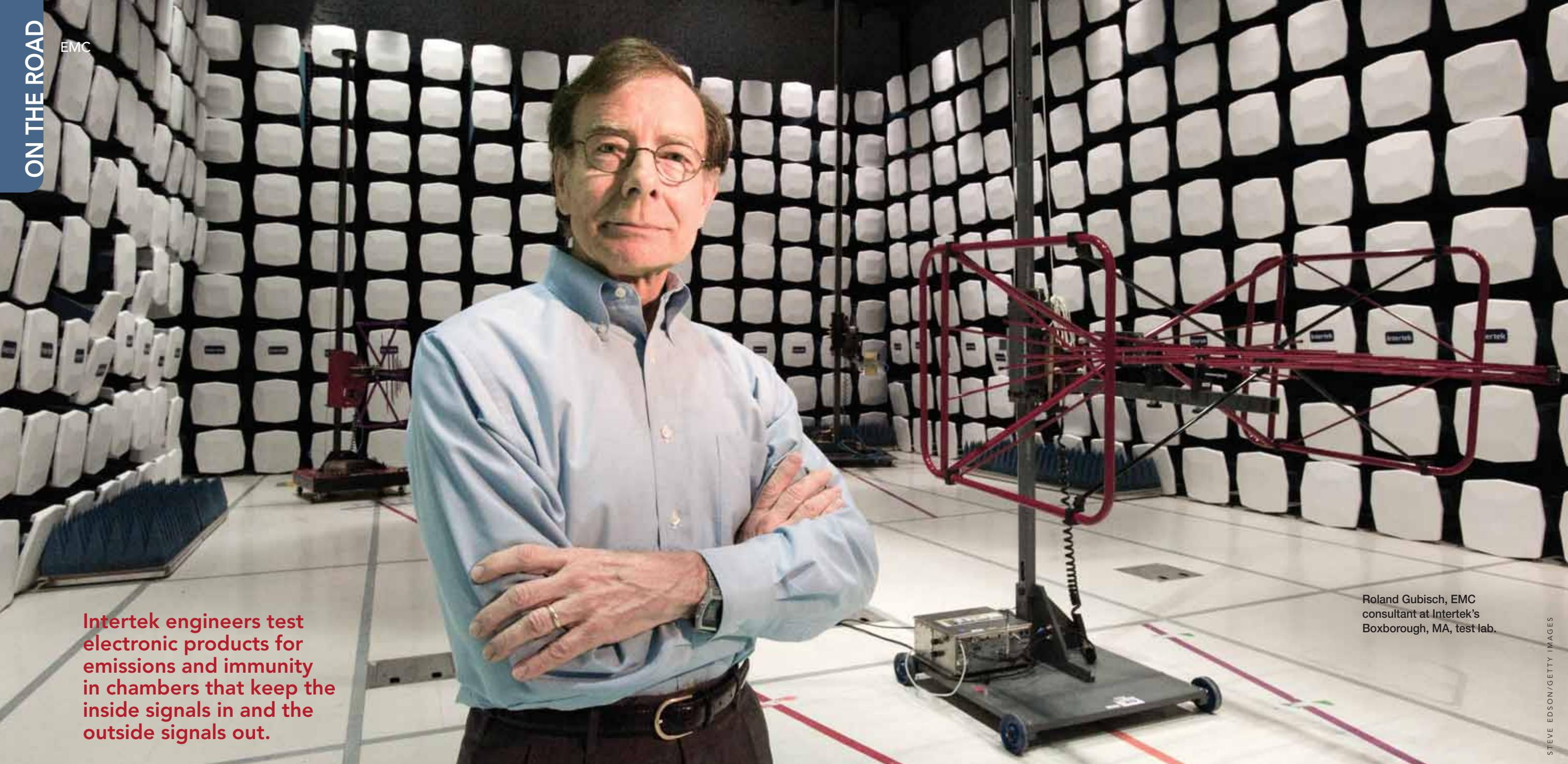
**Intertek engineers test electronic products for emissions and immunity in chambers that keep the inside signals in and the outside signals out.**
