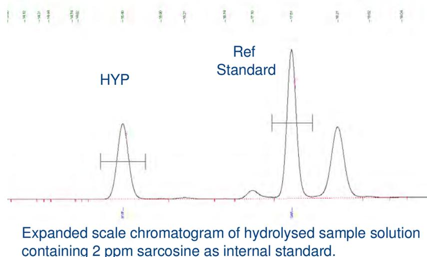
Expanded scale chromatogram of hydrolysed sample solution containing 2 ppm sarcosine as internal standard.
