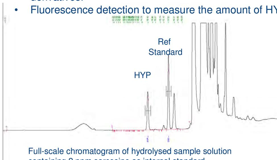
Full-scale chromatogram of hydrolysed sample solution containing 2 ppm sarcosine as internal standard.
