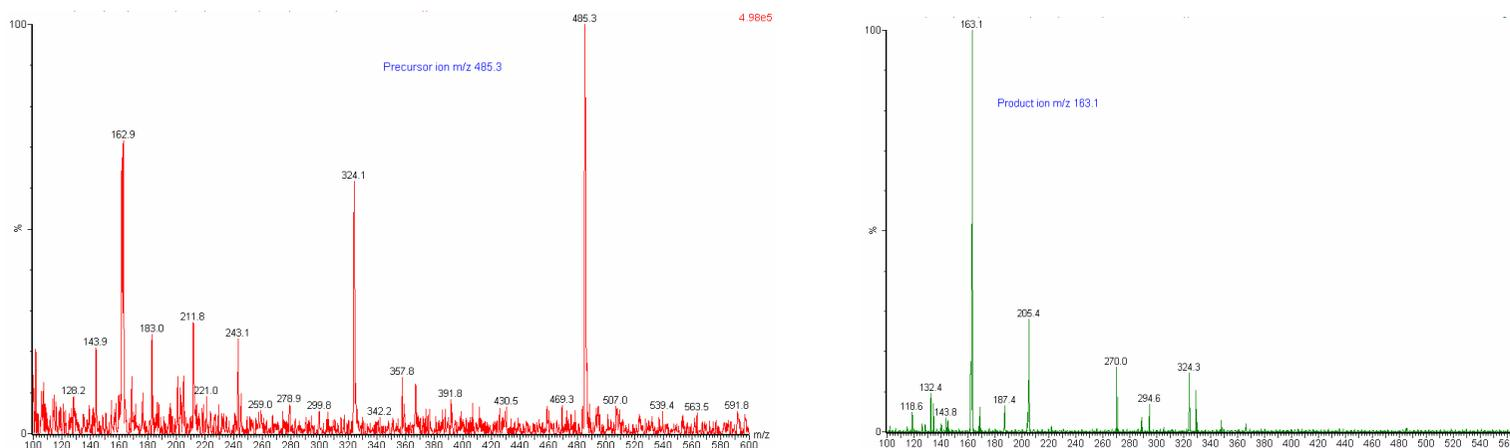
LC-MS/MS precursor and product spectra for kanamycin extracted from a processed collagen scaffold
