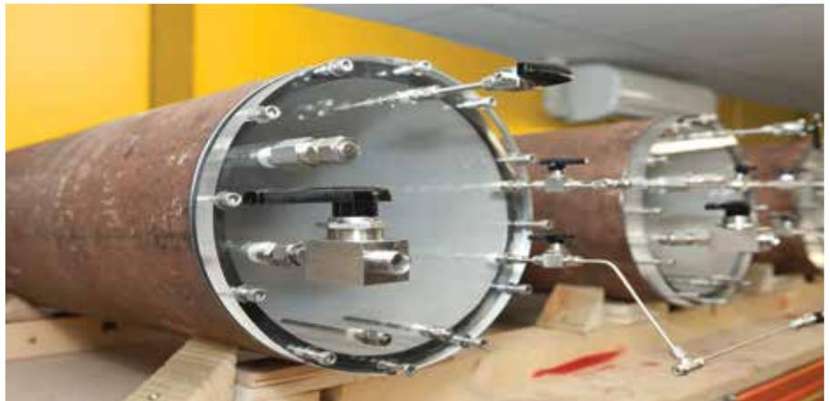
Pipeline during long-term wet lay-up
