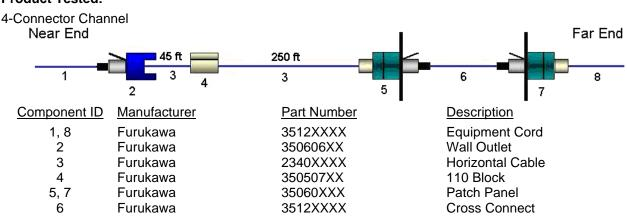
Standard(s)/Specification: ANSI/TIA-568-C.2 Category 6 with the applicable electrical transmission characteristics
