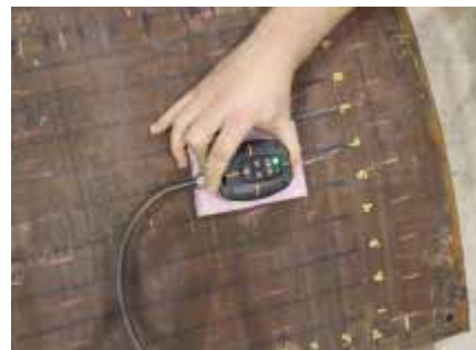
Figure 2: Example of a probe used on a shell with a 1-inch thick insulation
