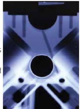
Digital radiographic image of a cylinder block
