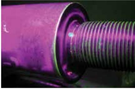
Crack on automotive shaft
