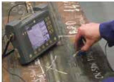
Manual ultrasonic testing of a plate
