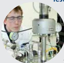
Carrying out corrosion fatigue testing in different aqueous environments is a standard procedure. This testing should take into account
