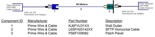
Standard(s)/Specification: ANSI/TIA-568-C.2 Category 6 with the applicable electrical transmission characteristics
