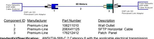
Standard(s)/Specification: ANSI/TIA-568-C.2 Category 6 with the applicable electrical transmission characteristics
