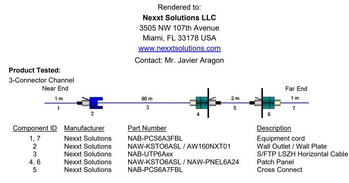
Standard(s)/Specification: ANSI/TIA-568.2-D Category 6A and ISO/IEC 11801-1 Class E<sub>A</sub> with the applicable electrical transmission characteristics
