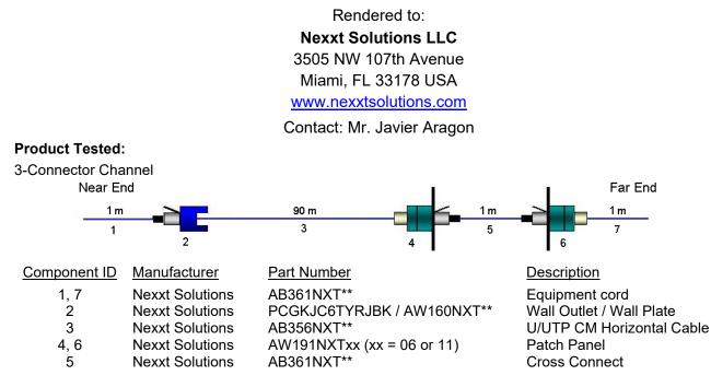
Standard(s)/Specification: ANSI/TIA-568.2-D Category 6 with the applicable electrical transmission characteristics
