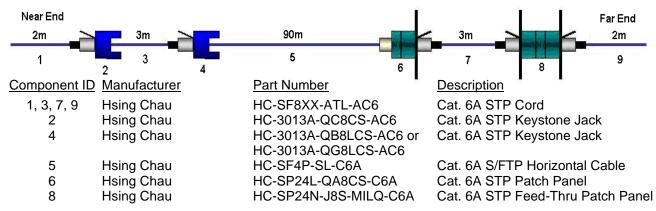
Standard(s)/Specification: ANSI/TIA-568-C.2 Category 6A with the applicable electrical transmission characteristics
