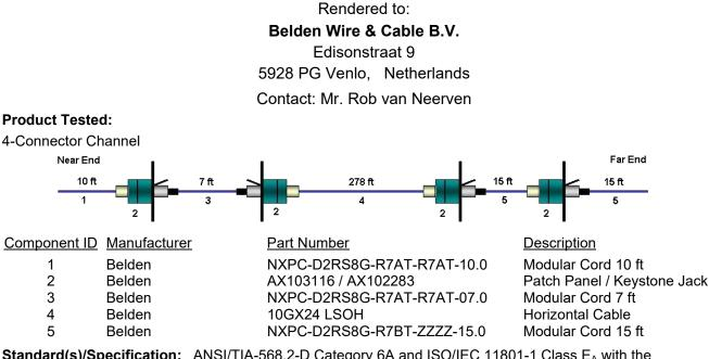
**Standard(s)/Specification:** ANSI/TIA-568.2-D Category 6A and ISO/IEC 11801-1 Class E<sub>A</sub> with the applicable electrical transmission characteristics
