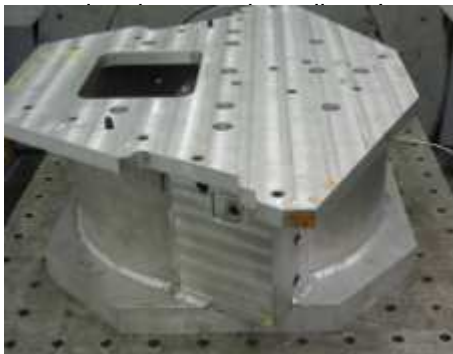
Front engine cover vibration fixture
