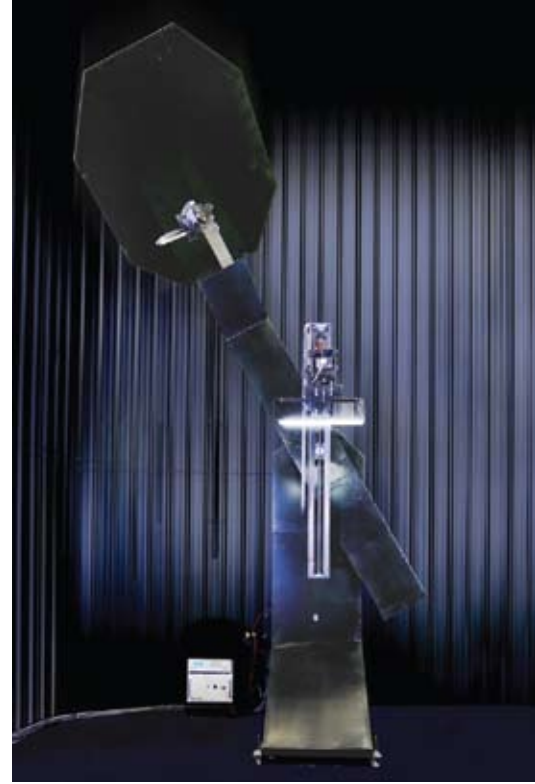
A Type C high-speed mirror goniophotometer for luminaire testing.
