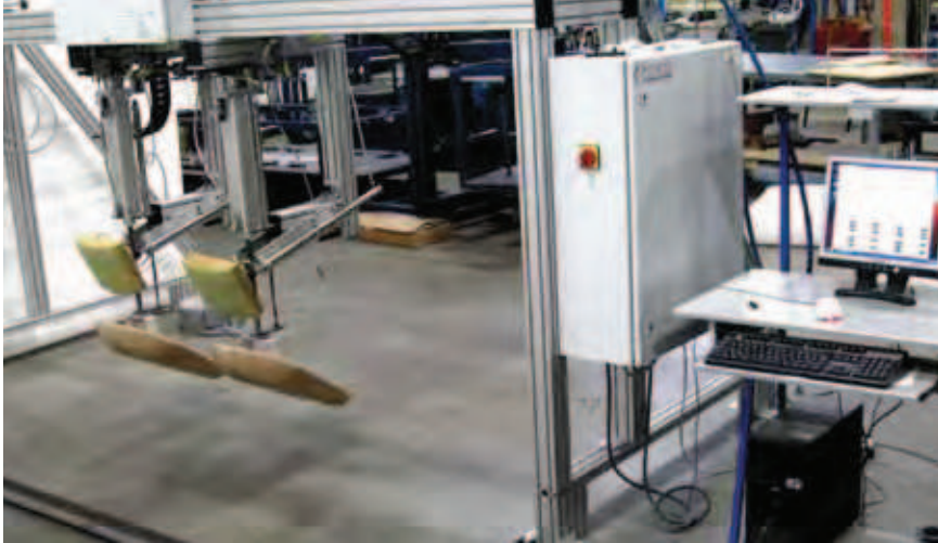
On the edge The BS EN1725 Section 7.5 standard is used to test the durability of a mattress edge.
