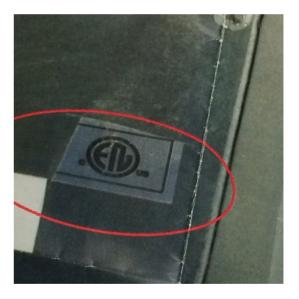
The counterfeit products can be easily identified by the separate ETL Certification Mark without a control number
