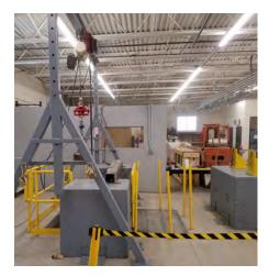
Intertek is pleased to announce our new Leading Edge testing capabilities. Leading Edge testing is a requirement of the ANSI Z359.14-2014 standard for personal fall arrest systems that are standard on many construction sites today. The test setup, which is located at Intertek's personal protective equipment lab in Cortland, NY, is the only accredited independent third party testing laboratory with these capabilities in North America.
