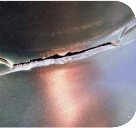
Crack at corner of a tank
