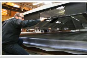
Roofing manufacturers want assurance that their roofing products have been tested to the highest possible rated pressure that they can achieve, and this service expansion provides that capability. For those looking to enter the Canadian market, the Coquitlam wind uplift chamber provides a fast and efficient pathway through certification to CSA A123.21.
