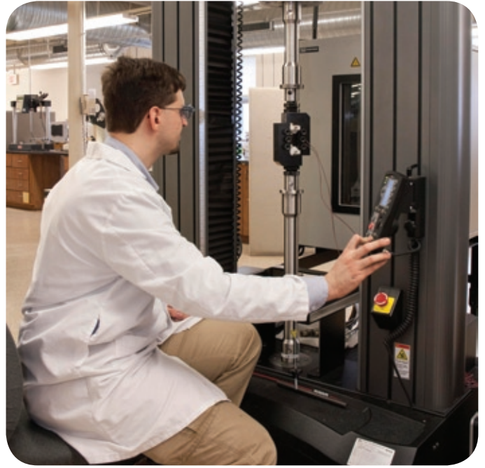
Composites Test Engineer performing V-notch Rail Shear for in plane shear properties.
