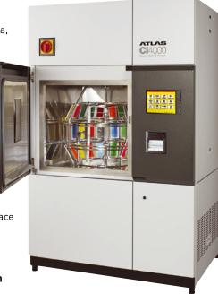
The latest Atlas sample holder can handle a wide range of specimens
