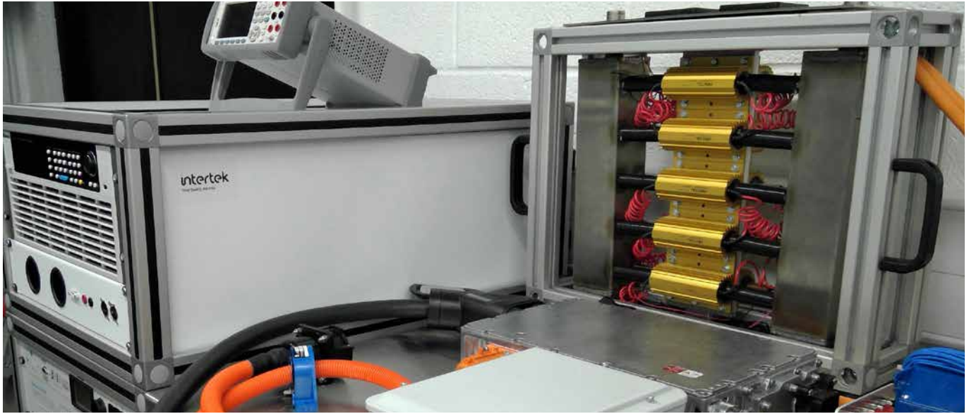
HV junction box undergoing dynamic load carrying test
