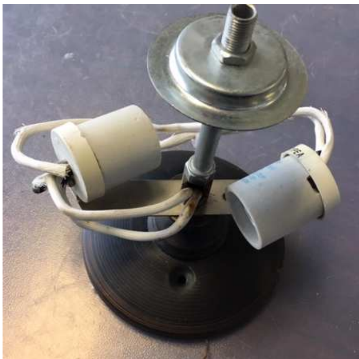
Insulated wiring routing (without lightbulbs) lens removed
