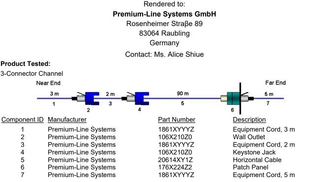
**Standard(s)/Specification:** ANSI/TIA-568.2-D Category 6, ISO/IEC 11801-1 Class E and IEEE 802.3btTM for support of Type 4 remote powering applications (PoE++) with the applicable electrical transmission characteristics
